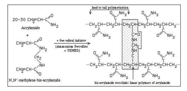
Acrylamide cross-linked by N,N'-methylene bisacrylamide. The polymerization is initiated by APS(ammonium persulfate) free radical,
